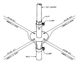
fig. 5. Detail showing attachment of top guys, "umbrella" wires and top loading whip.
